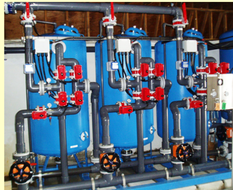
Skid Mounted With Carbon Steel Vessels and Automated Valve Harness
