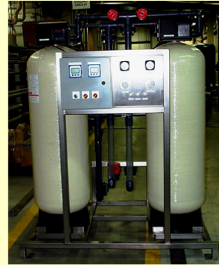
Skid Mounted with Composite Tanks and PLC
